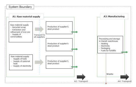
Figure 2. Simplified process tree.
